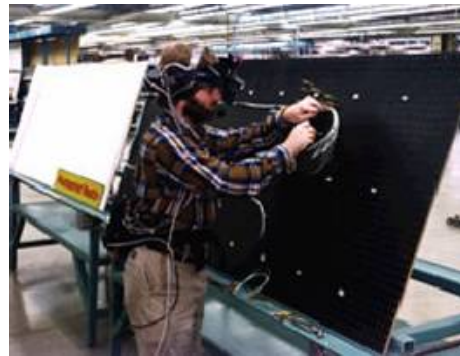
Figure 23: AR applied to maintenance work.
